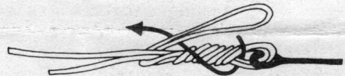
FIG. 2: Twist looped end 4 to 6 turns around main line (the easiest method is to hold both ends of line between thumb and index finger of one hand and roll hook shaft between thumb and finger of the other hand).
