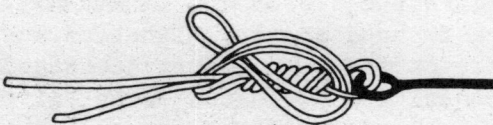
FIG. 3: Pass looped end of line through loop which hook is strung . . . then back up through big loop spanning knot.
