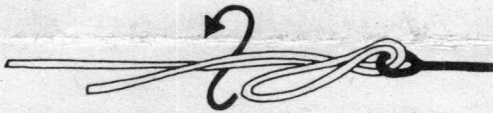
FIG. 1: Double 6 or 8 inches of your line and pass looped end half way through eye.
